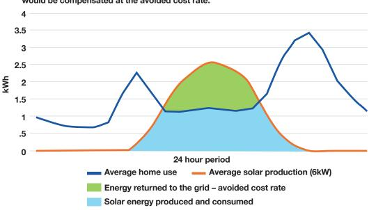
Energy produced and used by the consumer, shown in light blue, would be an energy offset at your retail rate. The area shaded in green is energy returned to the grid that would be compensated at the avoided cost rate.
