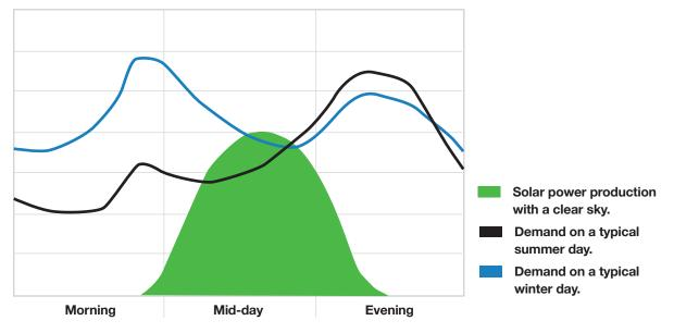
On a clear day (green curve) solar power generation does not match well with the time when your electric cooperative needs electricity the most.
